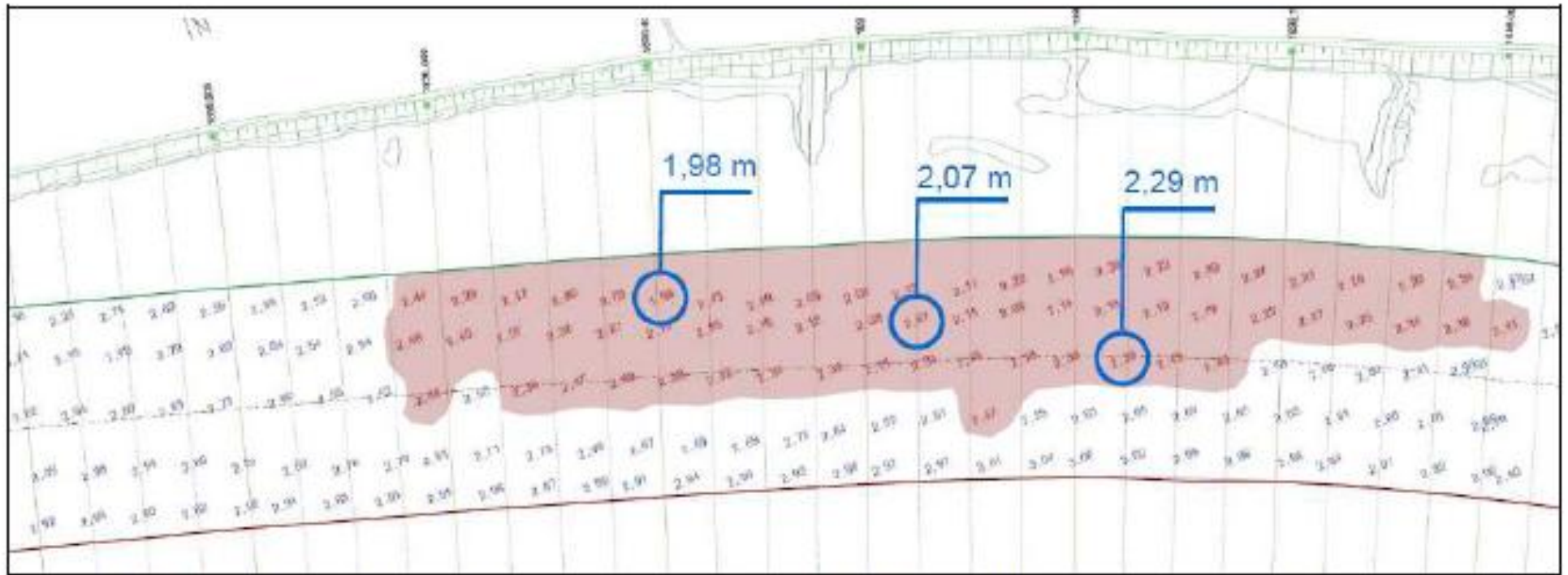
Figure 3.6: Track plot of fairway depth information of a shallow, available at the DoRIS website. Source: via donau.
