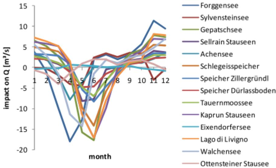
Fig. 4.1: Simulated impact of the reservoirs on discharges between 1991-2007.
