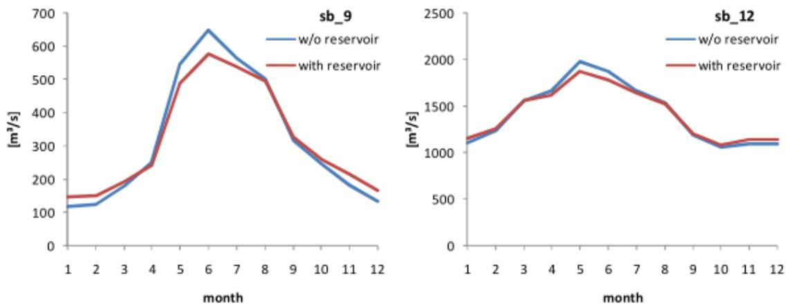
Fig. 4.2: Simulated discharge with and without influence of reservoirs within the period 1991-2007. (a) gauge Oberaudorf / Inn, (b) gauge Achleiten / Danube.
